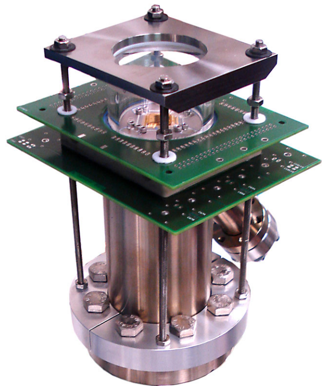
Fig. 6 Essential vacuum setup: a simple and compact custom made steel chamber with a CF 50 flange provides the basis for the chip holder, and provides an exit port for the laser beams through a CF 16 flange view port. On the polished surface of the tube, the ceramic chip carrier is placed, and on top of that a cylindrical glass cap with an interferometric quality window, anti-reflection coated for all our laser wavelengths. The chip carrier is connected to printed circuit boards (see Sect. 5). The multipin connectors are not shown. The whole stack is compressed with a steel frame by threaded rods
