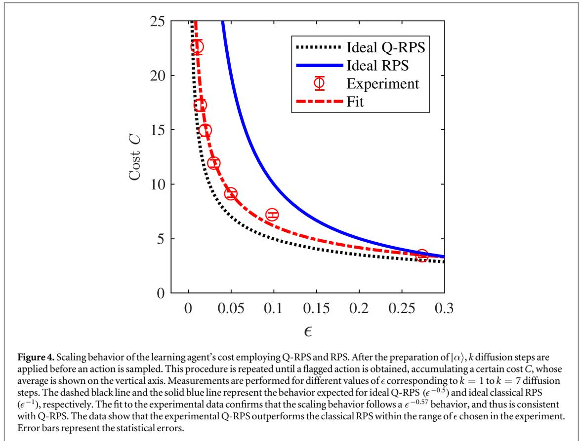
expected classical RPS, and clearly outperforms the classical RPS, as shown in figure 4. The deviation from the ideal behavior is attributed to a small detuning of the RF pulses implementing coherent operations, as we discuss in section 4.1.
