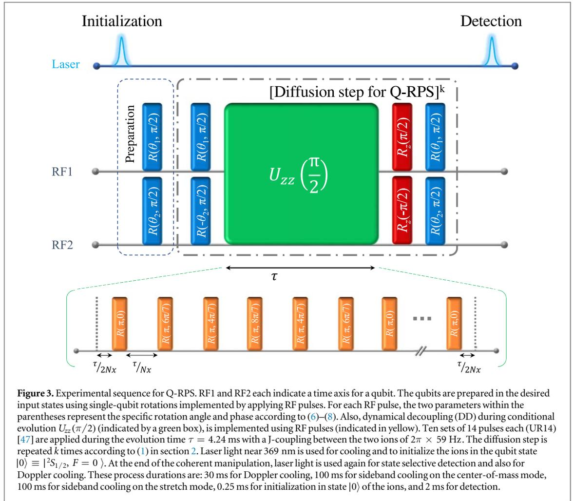
coherence time. Such a long coherent interaction time is accomplished by the DD pulses applied to each qubit simultaneously.
