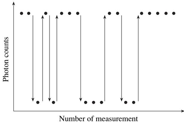
**Fig. 2.** Trajectory of the results (light scattering “on” or “off”) of subsequent individual measurements. On-off pairs represent excitation (of the atom) and absorption (of the drive radiation), off-on pairs de-excitation and emission.
