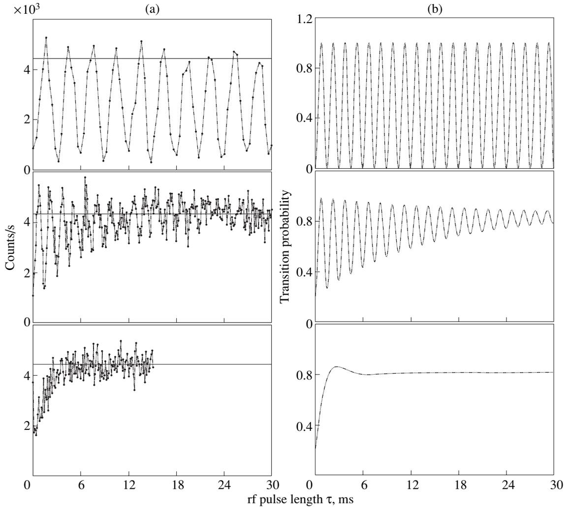
**Fig. 6.** Scattered-light response vs. length of microwave driving pulse. (a) Observed, with level of light applied to the ion *during* the drive: no light (top), 2 nW (middle), 20 nW (bottom). (b) Simulated: Rabi frequency  $\Omega_L = 0$  kHz (top), 50 kHz (middle), 500 kHz (bottom).
