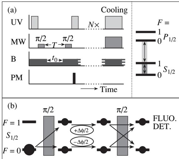
**Fig. 3.** Gating scenario of double-pulse driving by microwave (MW), UV probing, switching of magnetic field B, and detection of scattered light (PM), and simplified level scheme of atom (top). Interpretation as atomic-wave Mach-Zehnder interferometer in configuration space (bottom). The beam splitters are represented by the two  $\pi/2$  driving pulses.
