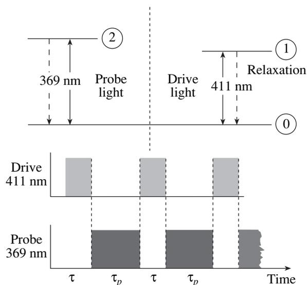
**Fig. 1.** Double-resonance addressing of individual atoms by alternating drive and laser probe pulses that excite resonance scattering to be detected. Here the driving pulses are laser light, and the wavelengths correspond to the ion  $^{172}\text{Yb}^+$ .
