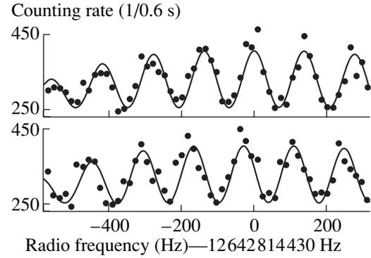
**Fig. 4.** Photo counting rate of single-ion fluorescence vs micro-wave detuning. Each data point shows accumulated results of 300 attempts; dc magnetic field  $B_0$  constant (top), and set to  $B_0 - \Delta B$  during  $t_0$  yielding the phase shift of fringes  $\langle \Delta\phi \rangle = 1.28$  rad. (From [4].)
