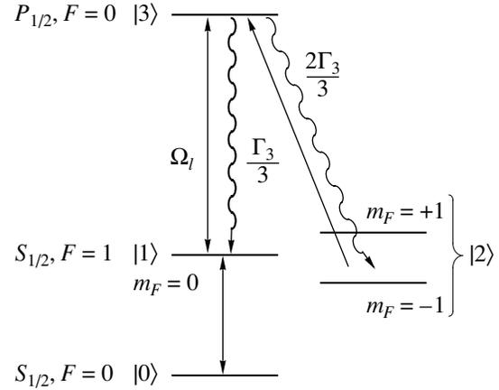
Fig. 7. Simplified level scheme of the  $^{171}\text{Yb}^+$  ion used in the described microwave-optical double resonance experiment.
