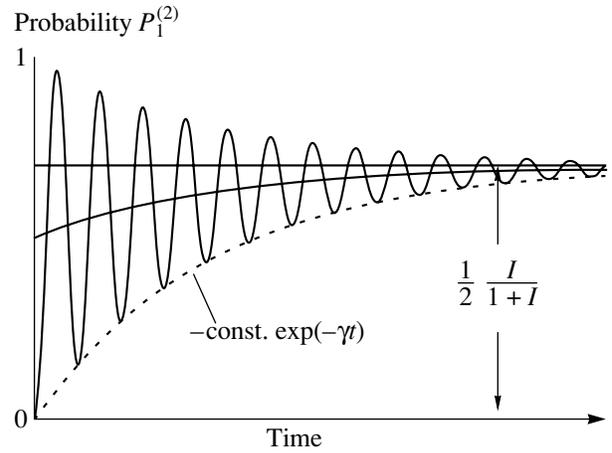
Fig. 8. Probability of upper-state (1) population, vs. time, of a relaxing atomic two-level system [13]. The evolution is characterized by the decay of the nutational oscillation ( $\gamma$ ), and by level of saturation determined by  $I = \Omega^2 / \Gamma \gamma$ .
