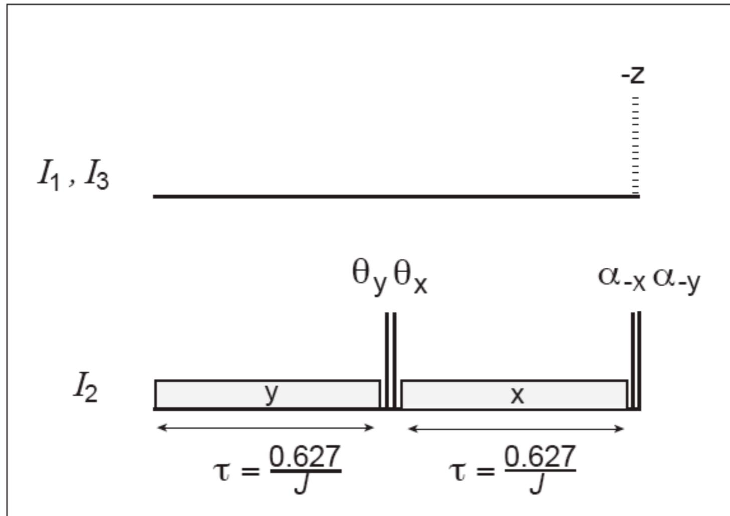
$\theta = 180^\circ - \alpha = 31.4^\circ$ , weak pulse amplitude:  $0.52 J$
