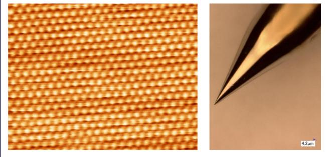
Scanning tunneling microscopy (STM) allows the characterization of surfaces on the atomic scale. The tip of the STM is the most important and most delicate part, and its preparation is crucial for all measurements. In this project, an existing setup for tip preparation will be optimized with the goal of a routine fabrication of reliable tips for our ultra-high vacuum microscopes.
