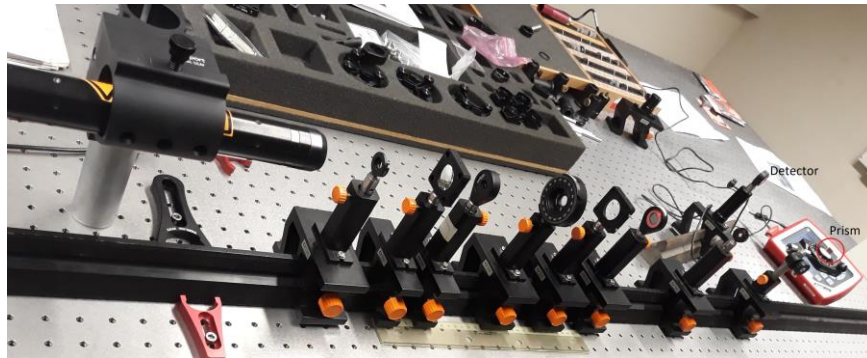
Figure 9. Optical setup for directly measuring the plasmon extinction.
