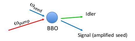
Generation of IR pulses from fs Ti:Sa 800 nm laser output.
