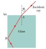
In figure left , a light ray enters a glass slab at point A at incidence angle  $\theta$ =45.0° and then undergoes total internal reflection at point B. What ist he minimum value fort he index of refraction of the glass can be inferred from this information ?
