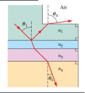
In the figure left, light is incident at angle  $\theta_1$ =40.1° on boundary between two transparent materials. Some of the light travels down through the next 3 layers of transparanet material., while some o fit refelects upwardsand then escapes into the air. If n<sub>1</sub>=1.30, n<sub>2</sub>=1.40, n<sub>3</sub>=1.32 and n<sub>4</sub>= 1.45, what ist he value of  $\theta_5$  in the air and of  $\theta_{14}$  in the bottom material?
