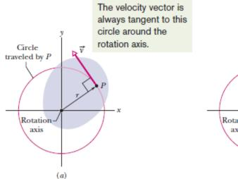
The acceleration always has a radial (centripetal) component and may have a tangential component.
