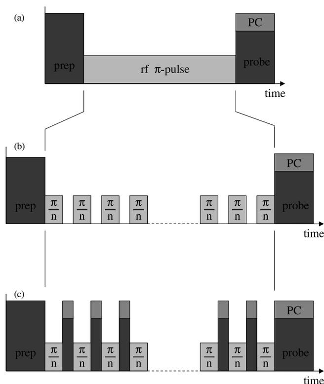
**Figure 8.** Scheme of measurement with (a) one driving  $\pi$  pulse, (b) with fractionated  $\pi$  pulse ( $n$ -times  $\pi/n$ ), no intermediate probing, and (c) with  $\pi/n$  pulses alternating with probe pulses. PC: photon counting.
